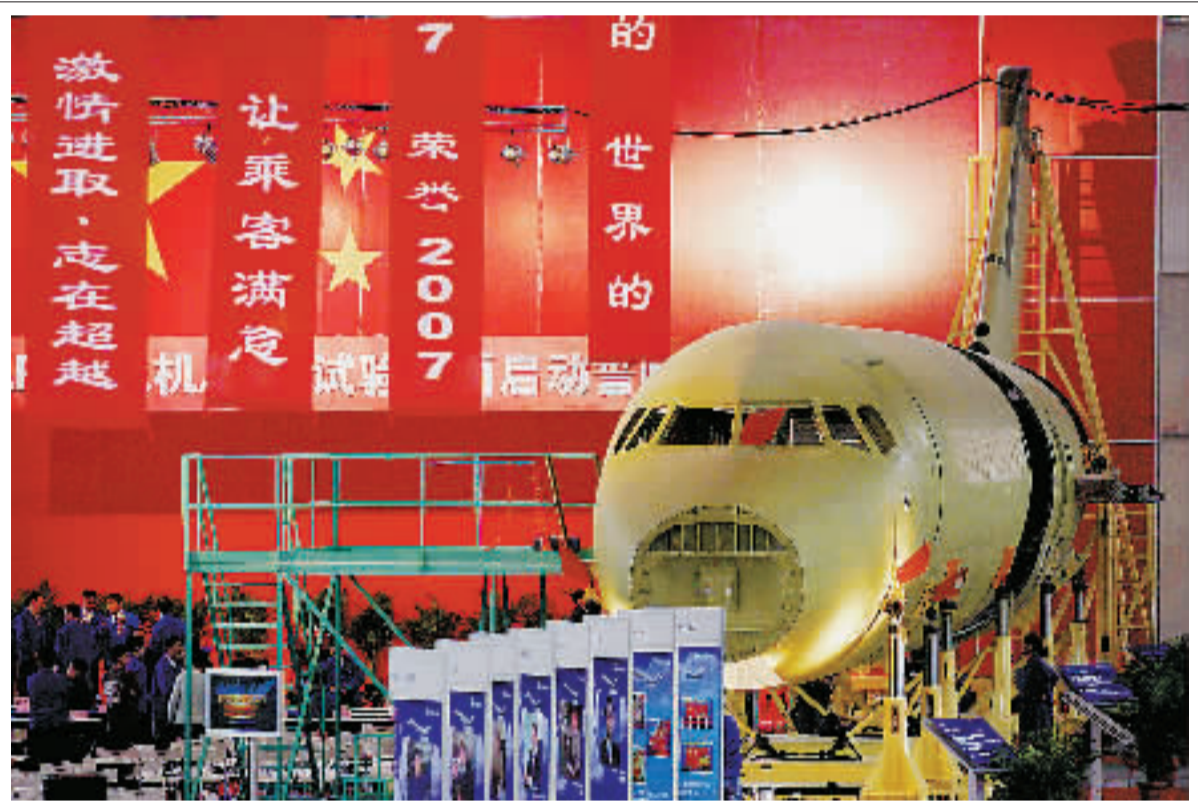
Final assembly of China's homemade regional jet with self-generated IPRs ARJ21 starting in Shanghai on March 30. The new airliner with passenger capacity ranging from 70 to 110 seats on different versions and wider cabin size in its class, is eligible to service short and mid range regional routes of over 80% current domestic routes (Courtesy: Newsphoto)
