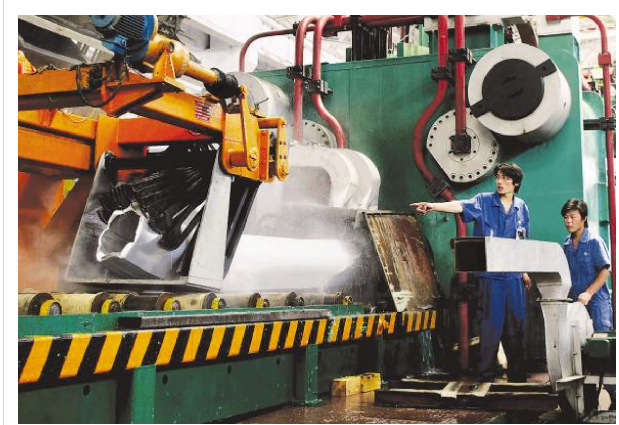
Shandong Longkou Conglin Group makes full use of its proprietary technology of aluminum profile pressing machine of 10,000 tons to develop new aluminum alloy for trains as well as for defense equipments, aviation and astronautics.
